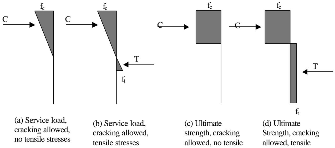
Figure 4- Various Models of Masonry Arch Ring Limit States
