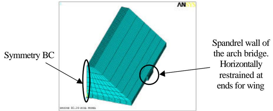
Figure 7- Half-Soil Model for Bridge #1
