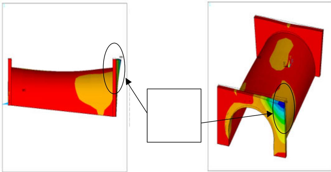
Figure 9- Deflected Shape of Bridge #3 under 315k Car Loading
