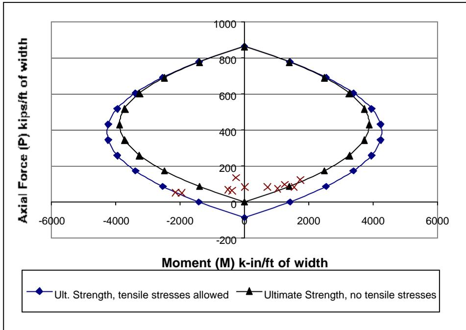
Figure 6- E-Rating Plot for E600 loading, Concrete Arch Bridge
