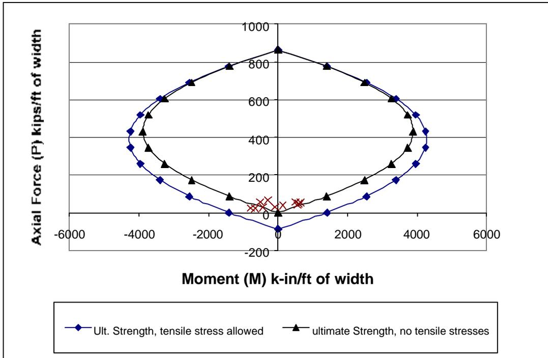
Figure 5- E-Rating Plot for E80 loading, Concrete Arch Bridge
