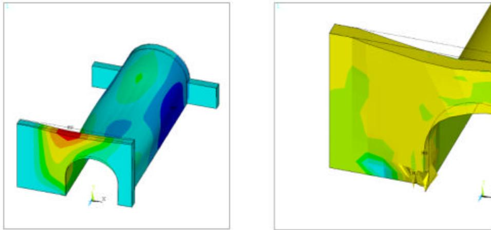
Figure 8- Deflected shape and Collapse on Bridge #2 ( $f'_c=125$  psi)
