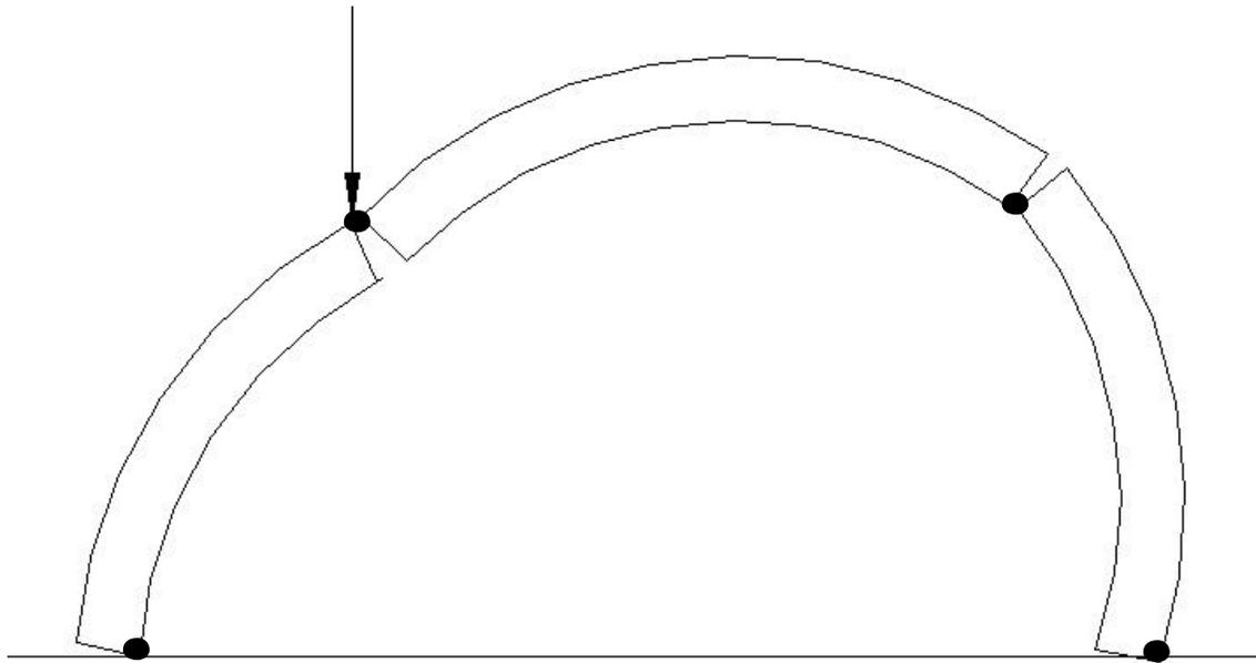
Figure 1- Collapse Mechanism of an Arch Bridge under Concentrated Load
