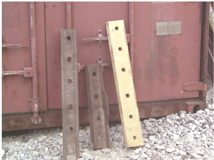
Figure 3-8 Conventional Bar, Compromise Bar & Insulated Joint Bar – Photo by J. E. Riley
